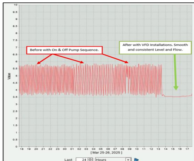
Flow trend showing before and after VFD installation
