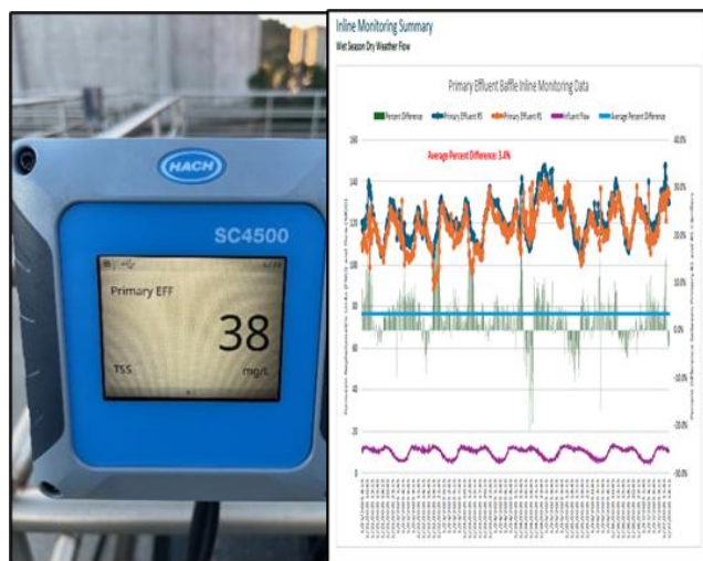
TSS meter showing mg/L value and TSS data trends
