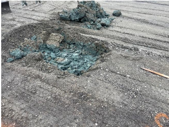
Unstable clay layer underneath the pavement
